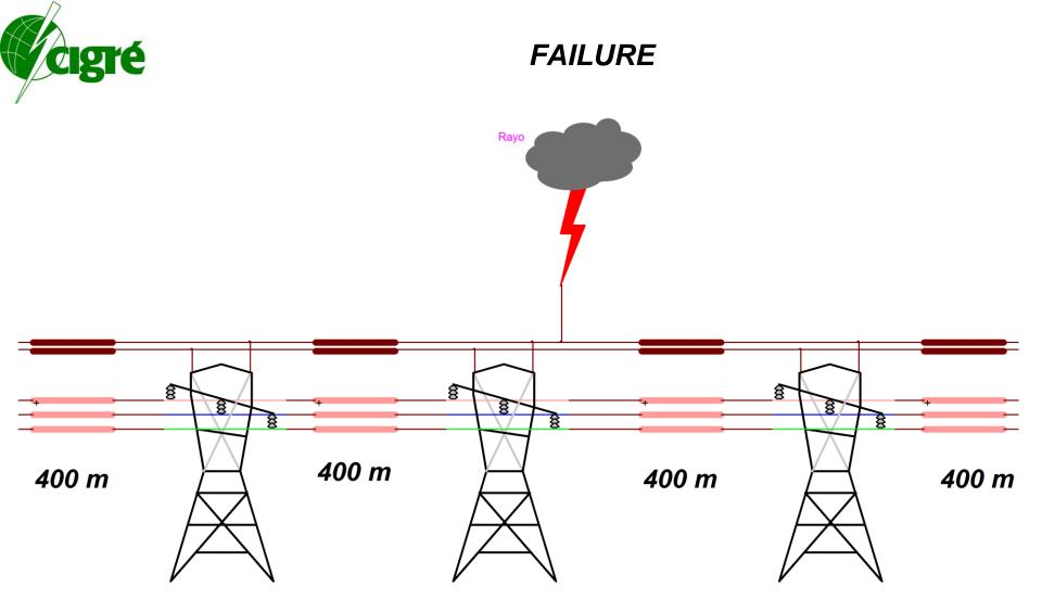
The situation presented to the lightning strike on one of the ground wires, resulting finally in a single-phase fault between a phase and structure of the tower.
