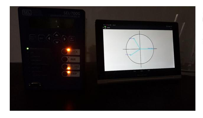
Mobile testing reading voltage phasors from an IED using a MMS client installed on a Tablet.
