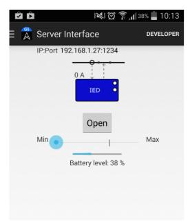
Sends the battery level of the mobile device via MMS on a BATT logical node.
